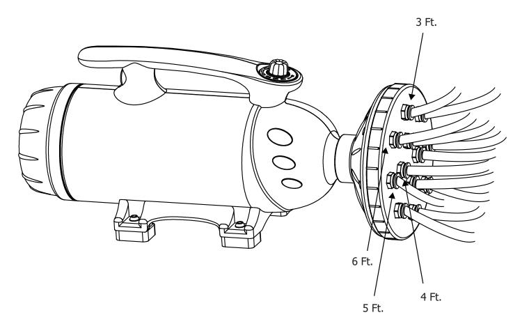
In order to achieve the maximized air pressure for wall drying, VIKING Equipment recommends that the  $1/2 \times 1/3$  inch hose be cut as shown above. Hoses beyond the suggested lengths above may result in a loss of pressurized drying capability. Pressure can be equalized or increased by connecting unutilized drying nozzles with unused hose.
