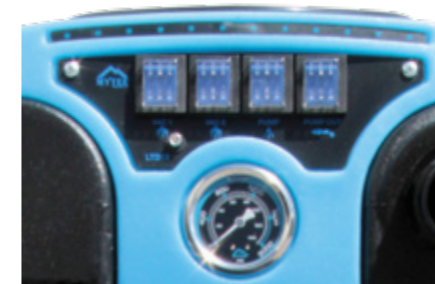
Switchplate featuring dual circuit indicator light strip.
