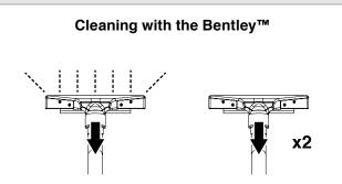
We recommend one wet pass followed by two dry passes. If using a heated extractor, this allows the machine to heat up more solution.
