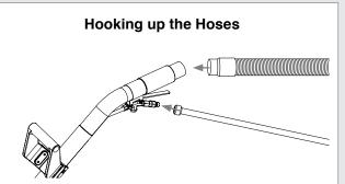
After the Vacuum Hose and Solution Hose are attached to the extractor, connect the Solution Hose to the Male Quick Disconnect, and the Vacuum Hose to wand tube.
